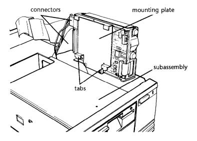
Notice that there are two tabs facing downward on the bottom of the mounting plate. These tabs will fit into two slots in the right side of the subassembly.
